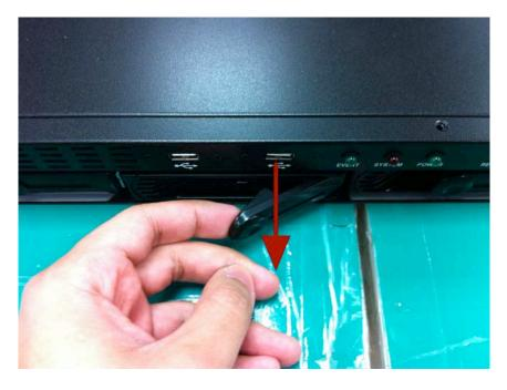
Release the HDD tray by pulling the latch.
